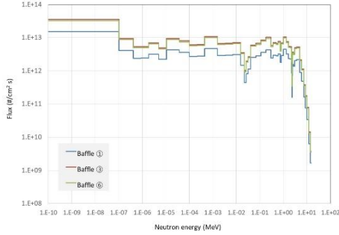
Fig. 2. Neutron spectra for baffle plates at three locations
