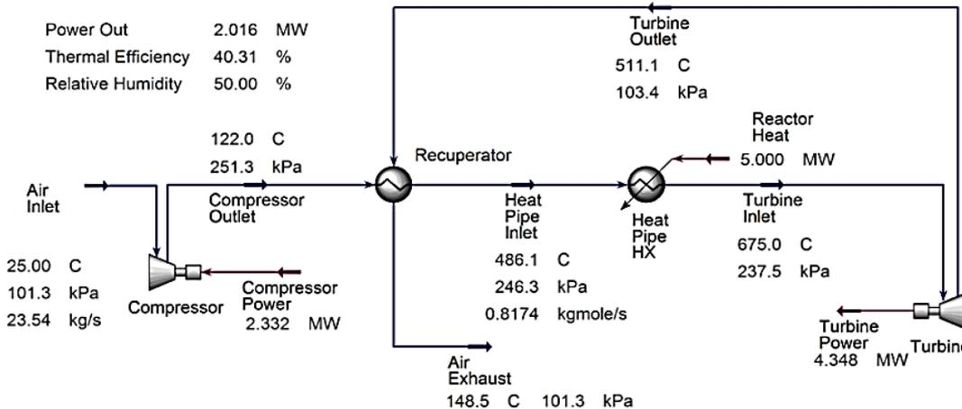
**Fig.** Aspen HYSYS model of heat recuperated air Brayton cycle [9].
