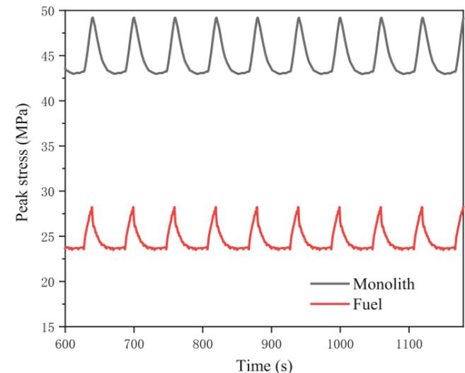
Fig. The stress oscillation for geyser boiling condition [3].
