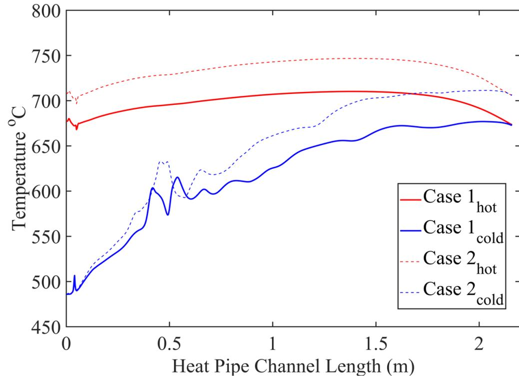
**Fig.** Temperature distribution of hot and cold sides via the channel length for both scenarios.
