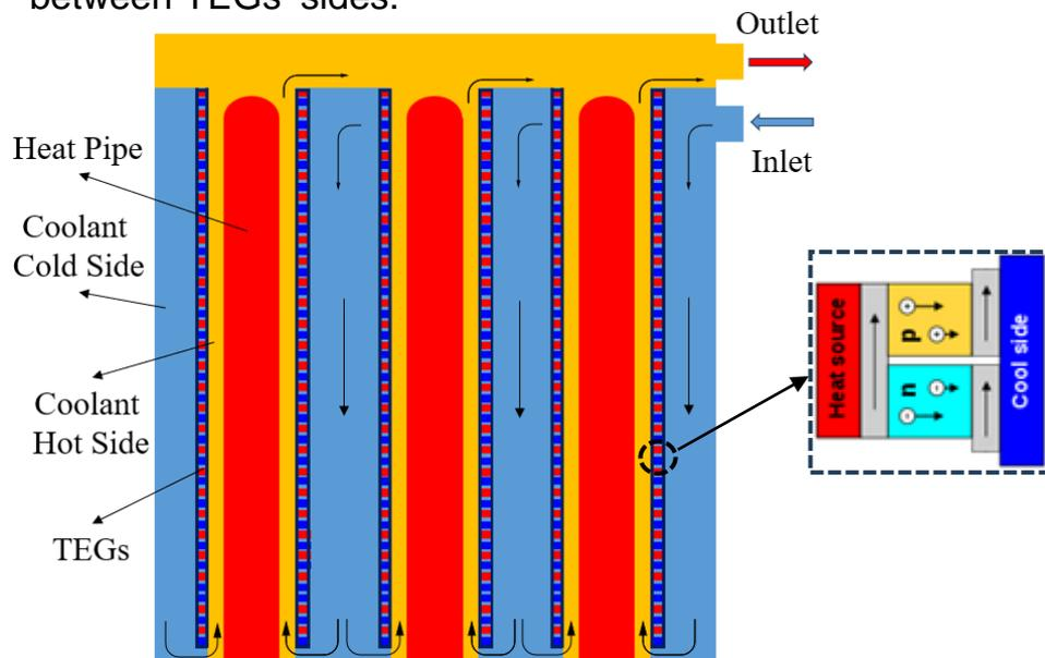
Fig. Simplified cross-sectional model of hybrid heat exchanger.
