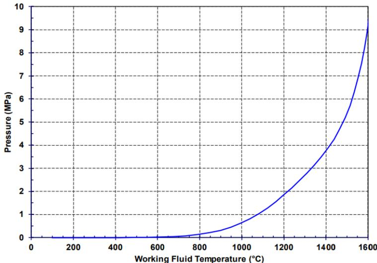
Fig. Potassium Equilibrium Pressure Temperature Curve [8].
