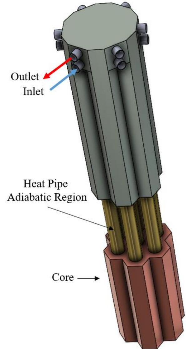
Fig. 3D representation of the design featuring seven heat pipes.
