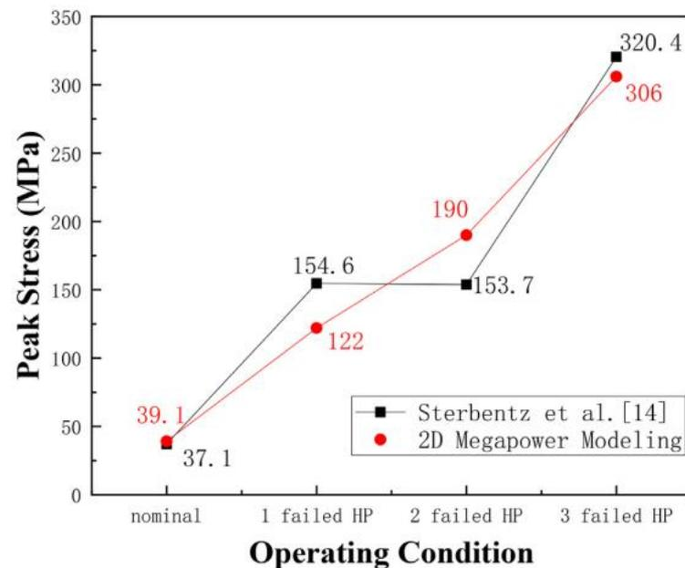
Fig. Peak stresses predicted by the 2-D and 3-D models [4].
