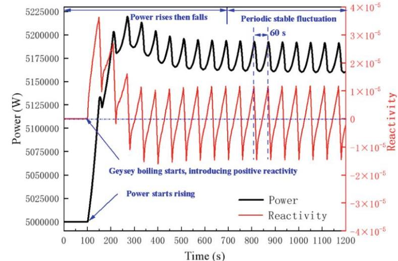
Fig. The effect of temperature oscillation on the core [3].
