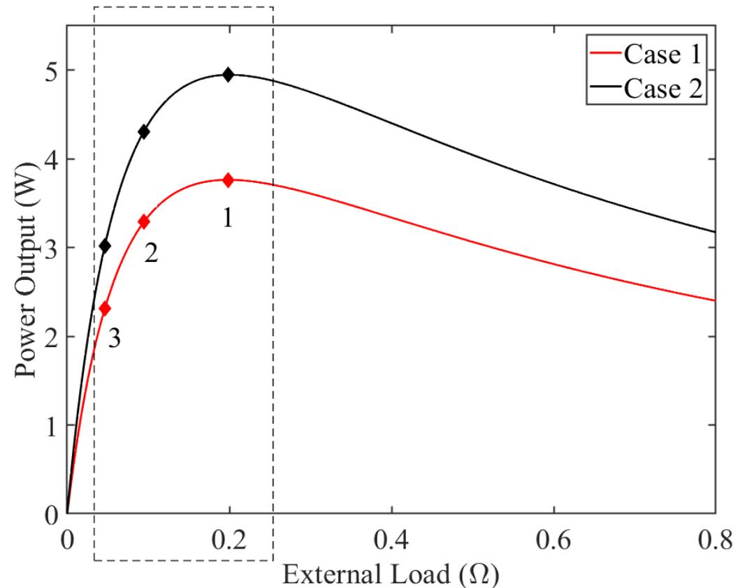
Fig. External load effect on power output of both cases.
