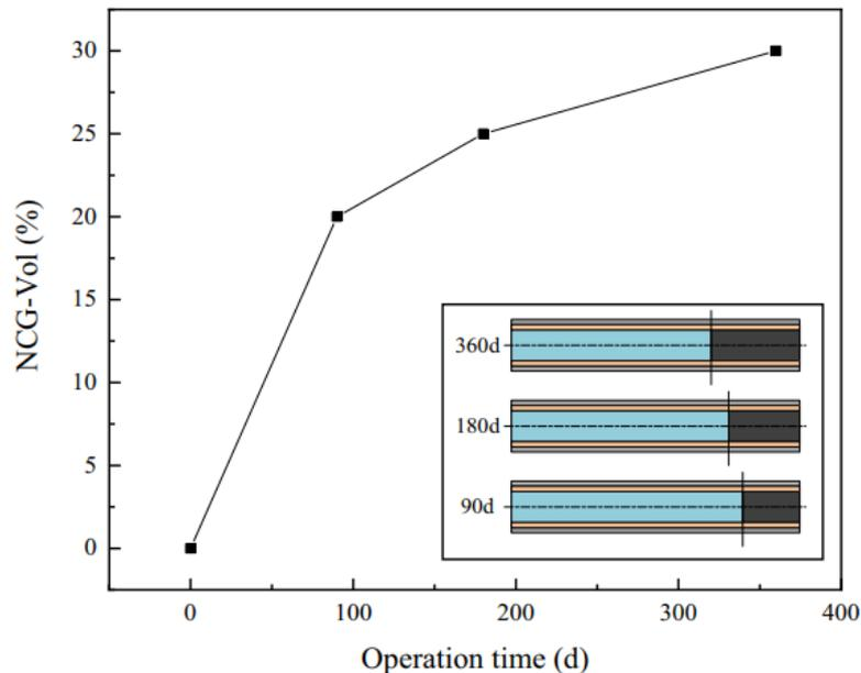
Fig. Change in NCG-vol during one year of operation [6].
