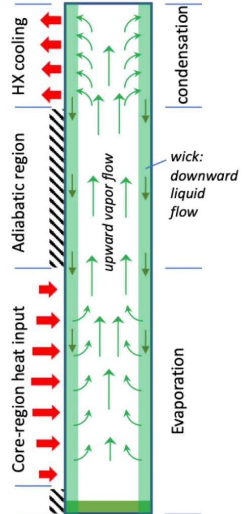
Fig. Illustration of a vertically oriented heat pipe [1].
