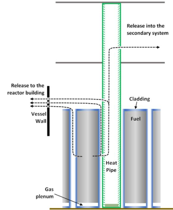
Fig. HP failure pathways [8].
