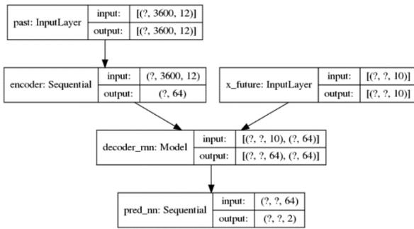
Fig. 2. Encoder-Decoder Model
