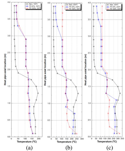
Fig. 3. Axial temperature distribution result for horizontal position (a)  $T_{\text{heater}} = 150^{\circ}\text{C}$  (b)  $T_{\text{heater}} = 200^{\circ}\text{C}$  (c)  $T_{\text{heater}} = 250^{\circ}\text{C}$
