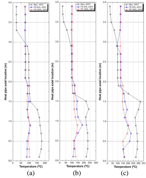
Fig. 2. Axial temperature distribution result for vertical position (a)  $T_{\text{heater}} = 150^{\circ}\text{C}$  (b)  $T_{\text{heater}} = 200^{\circ}\text{C}$  (c)  $T_{\text{heater}} = 250^{\circ}\text{C}$
