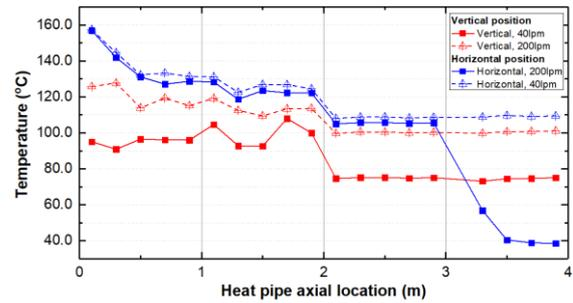
Fig. 5. Axial temperature distribution comparison for different cooling capacity and the orientation.
