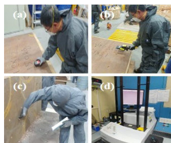
Fig 2. (a) Dose rate test, (b) Surface contamination measurement (Direct method), (c) Surface contamination measurement (Indirect method), (d) Low background alpha/beta counting system
