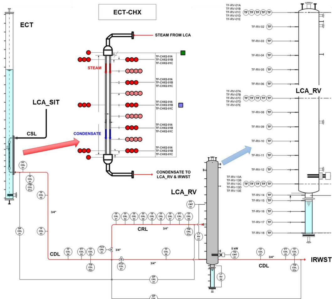
Fig. 1. Schematic diagram of SISTA2 with temperature measurement points (from CHX to LCA\_RV and IRWST)
