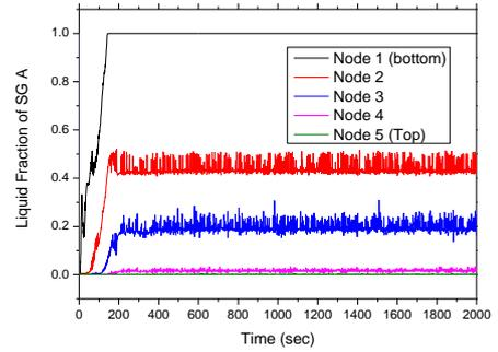
Fig. 10. Liquid fraction of SG A (57 kg/s)
