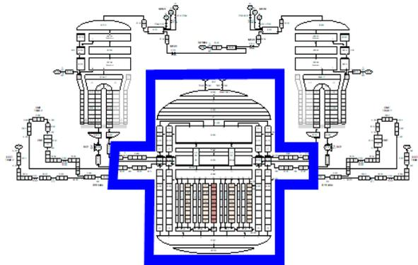
Fig. 1. MARS Nodalization of BANDI-60S
