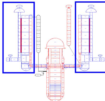
Fig. 3. Nodalization of Helical tube steam generators
