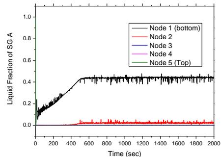
Fig. 5. Liquid fraction of SG A (52 kg/s)
