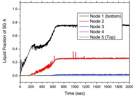
Fig. 6. Liquid fraction of SG A (53 kg/s)
