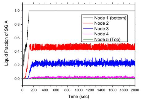
Fig. 11. Liquid fraction of SG A (58 kg/s)
