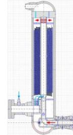
Fig. 2. Types of Helical tube steam generators
