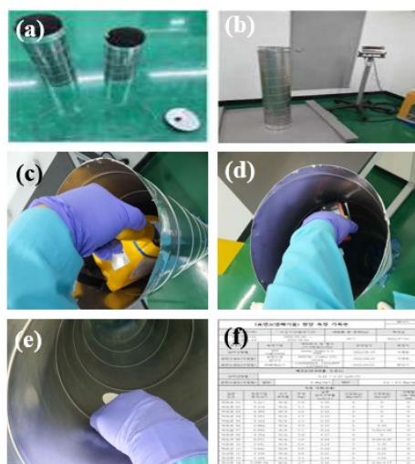
Fig 2 (a) surface area, (b) weight. (c) surface contamination (direct method), (d) surface radiation dose rate, (e) surface contamination (indirect method), (f) measurement record.
