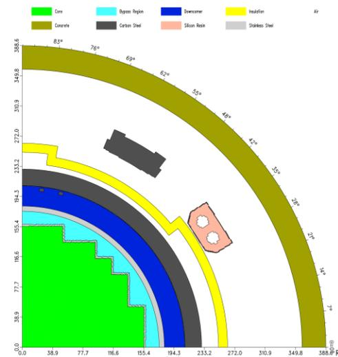
FIG. 1–[r,  $\theta$ ] model of the Ulchin Unit 4 reactor
