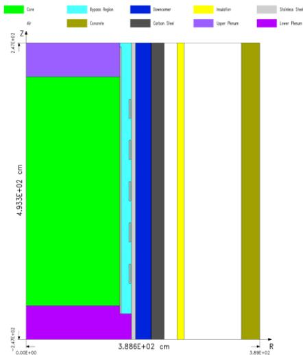
FIG. 2–[r,z] model of the Ulchin Unit 4 reactor
