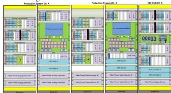
Fig. 2. Cabinet Configuration of the Test Facility
