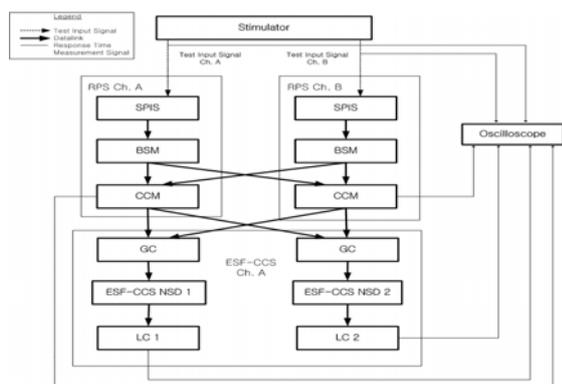
Fig. 4. Block Diagram of the Performance Test
