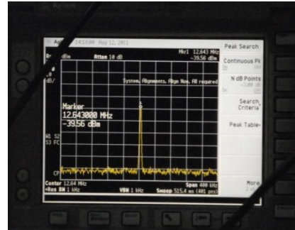
Fig. 7 The resonance peak of RF signal
