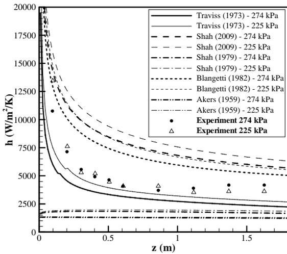
Fig. 1. The prediction of the correlations of condensation heat transfer coefficient with the experimental data of Henderson et. al. [3]
