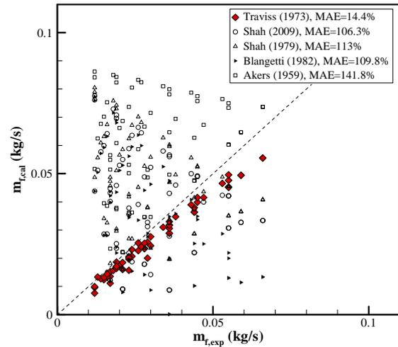
Fig. 3. The prediction of the condensation mass flow rate with the experimental data of Kim [4]
