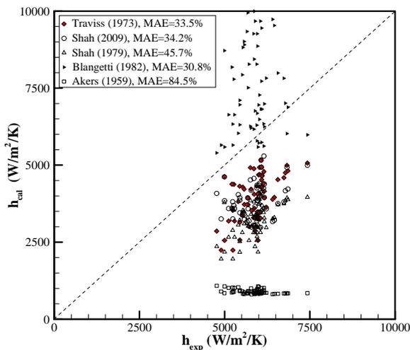
Fig. 2. The prediction of the correlations of condensation heat transfer coefficient with the experimental data of Kim [4]
