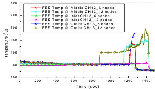
Fig. 4 Channel 13 FES Temperature Comparison vs. Node Number
