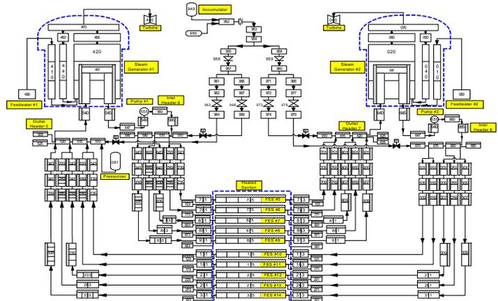
Fig. 1 MARS-KS Nodalization for RD-14M Facility
