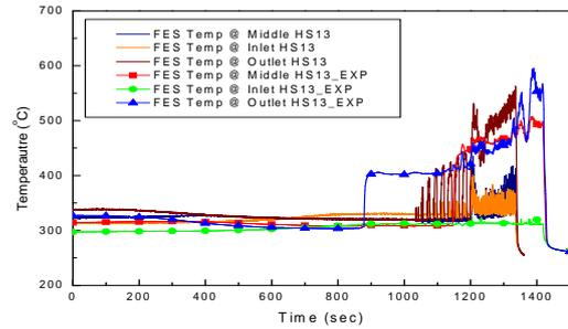
Fig. 3 Channel 13 FES Temperature
