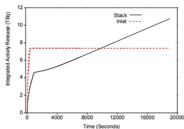
Fig. 5. Integrated I-131 release for LOCI
