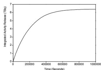
Fig. 6 Integrated I-131 release for PLOD
