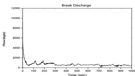
Fig. 2. Mass discharge from the break to inside containment
