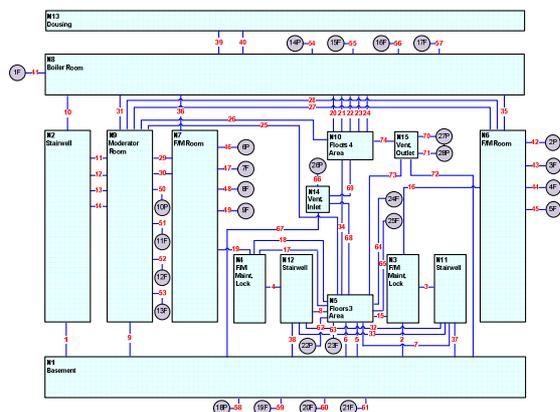
Fig. 1. Nodes and flow paths of the containment model
