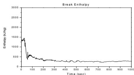
Fig. 3. Energy discharge from the break to inside containment
