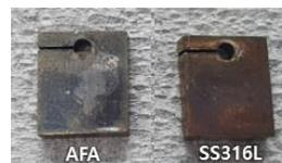
Fig. 2. LBE corroded DED-AFA and DED-316L specimens
