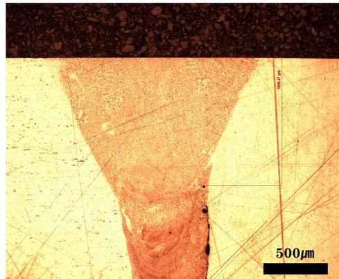
Fig. 6. Cross sectional microscopic image obtained in bead area
