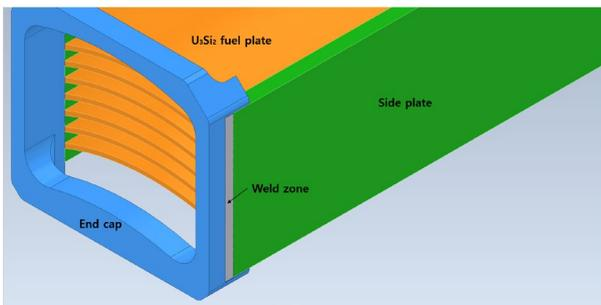
Fig. 1. Weld zone of KIMQI-GTA assembly
