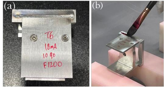
Fig. 5. (a) Welded test specimen and (b) Liquid penetration test for welded test specimen
