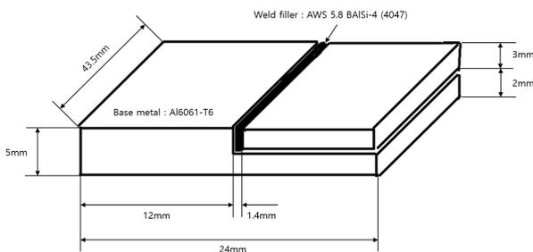
Fig. 4. Specimen size for EB welding test
