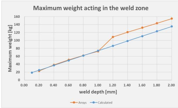
Fig. 3. Maximum weight on the weld area in function of the weld depth
