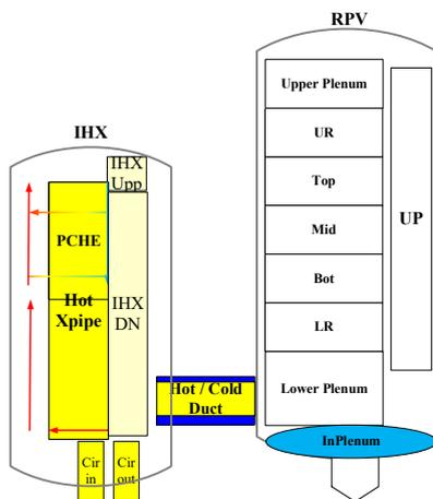
Fig. 1. MELCOR CVH model of VHTR350
