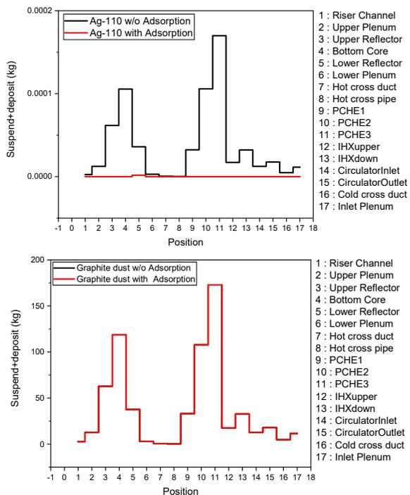
Fig. 3. Mass change in Ag-110m and graphite dust
