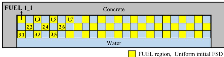
Figure 8. Checkerboard storage of assemblies
