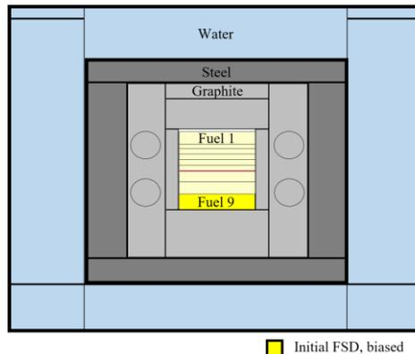
Figure 1. Vertical cross section of AGN-201K
