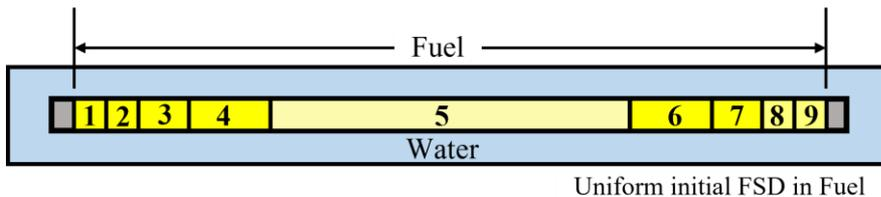
Figure 14. Pin-cell array with irradiated fuel
