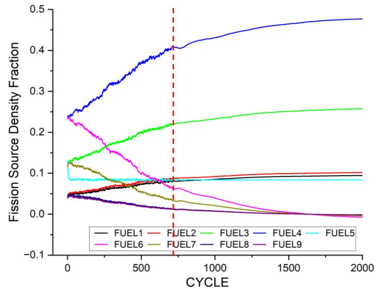
FSD fraction with Kalman filter after 700 cycle
