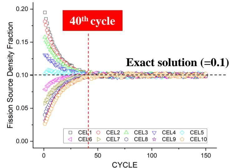
Figure 7. Fission source density fraction of slab
