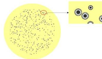
Fig. 1. TRISO particles in fuel pebble
