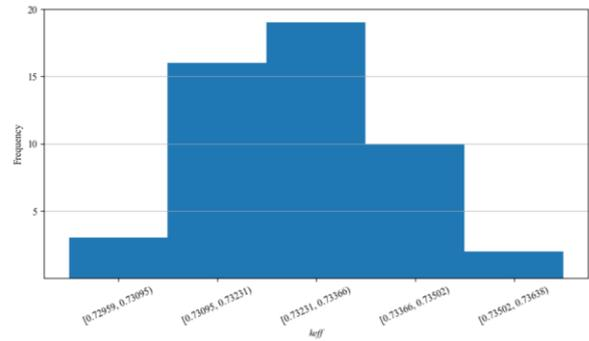
Fig. 5. Histogram of  $k_{eff}$  with a different selection of fuel and graphite
