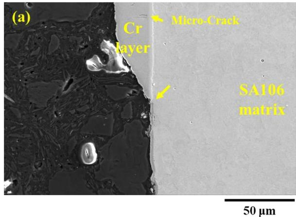
Fig. 3. The interface between Cr-coated at 50 °C and the carbon steel disk SEM photographs.
