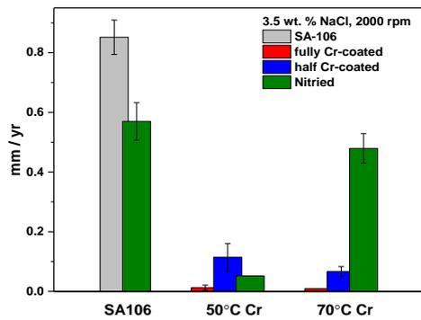
Fig. 1. Flow Accelerated Corrosion rate of as-received, Cr-coated, and nitrided SA106 disk calculated from FAC tests.
