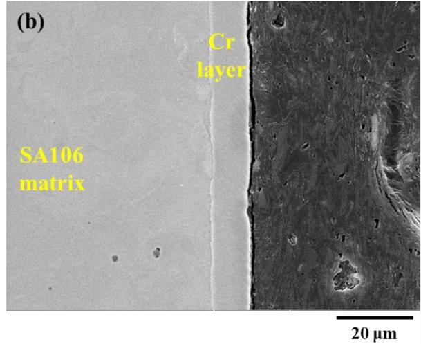
Fig. 2. The SEM cross-sectional photographs of Cr-electro-plated SA106 carbon steel at (a) 50 °C and (b) 70 °C.
