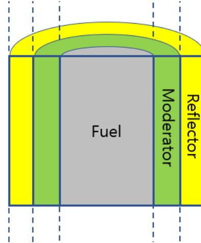
Fig 2. Infinite Cylinder Model for Side DF
