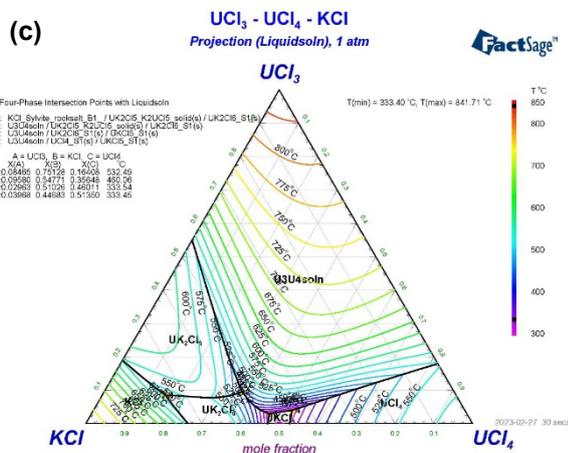
Figure 1. Projected ternary liquidus surfaces of  $UCl_3$ – $UCl_4$ –Base Salt systems (Base Salt: NaCl,  $MgCl_2$ , KCl).
