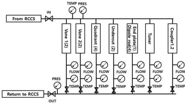
Fig. 3. Water-cooling system model of the RFQ cavity.
