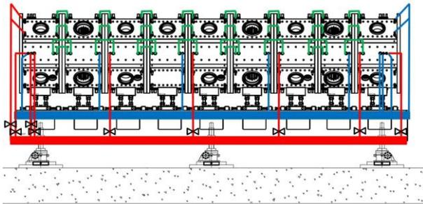
Fig. 4. Pipe connection of the RFQ cavity.
