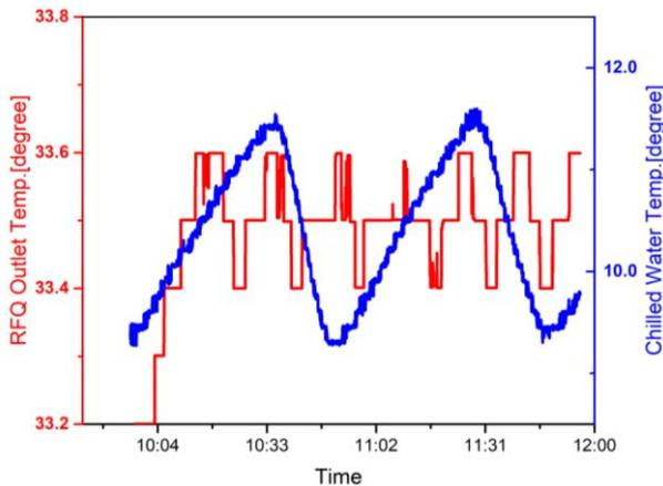
Fig. 5. Cooling water temperature at the RFQ cooling channel outlet and the chilled water temperature supplied by the convention facility
