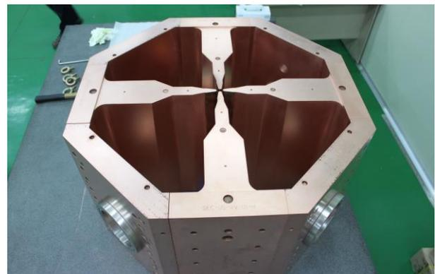
Fig. 2. RFQ cross-section of one of the nine sections. Holes for cooling channels in vanes and quadrants were plugged.
