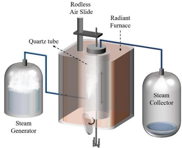
Fig. 1. Schematic of LOCA experiment facility.
