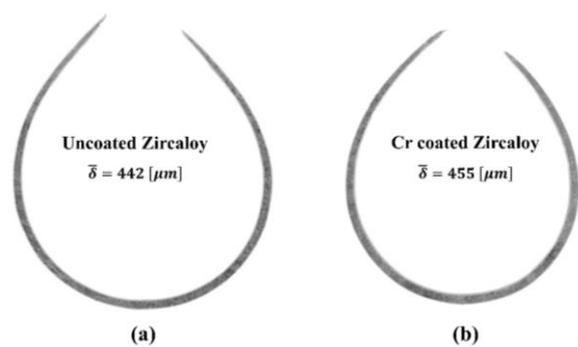
Fig. 4. Cross section of the thinned thickness of the specimens.
