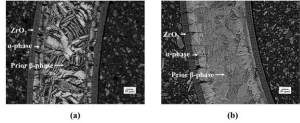
Fig. 3. Cross-section of oxidized specimen (WG-ECR = 17%) (a) Zircaloy-4 specimen (b) Zr-1.1Nb specimen.
