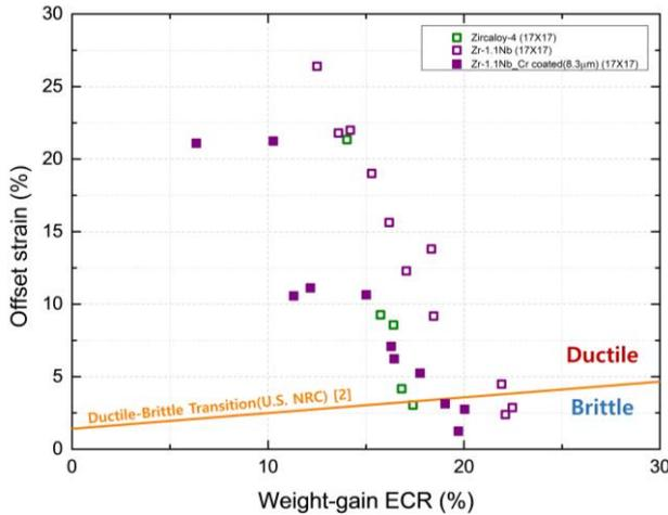
Fig. 2. Offset strain according to Weight Gain Equivalent Cladding Reacted (WG-ECR) and U.S. NRC criteria.
