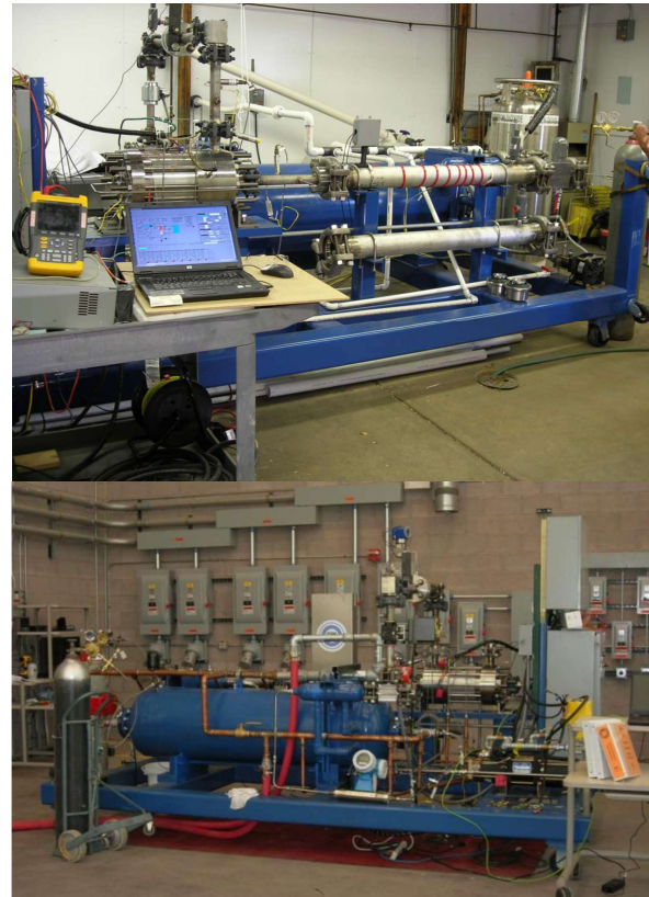
Fig 1. S-CO 2 Compressor Research Loop (Top : 2008, Bottom : 2011)
