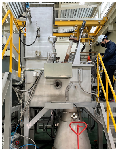
Fig. 1. Picture of 100kW plasma torch melting facility.
