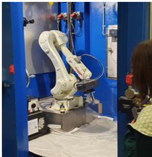
Fig. 1. Remote handling with a robotic arm at sample receiving cell.
