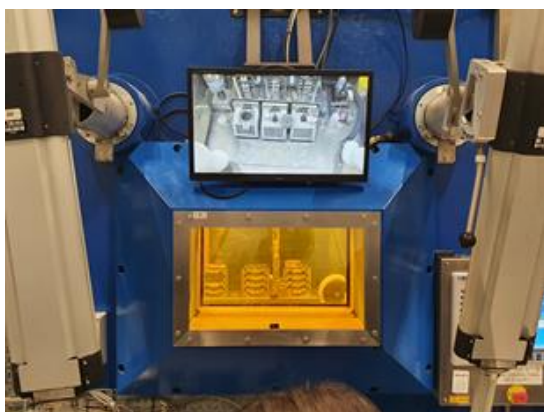
Fig. 2. Remote handling with both a radiation shielding window and a digital monitor of remote camera.
