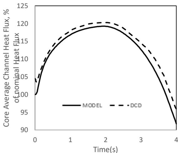
**Figure 6:** Average channel heat flux
