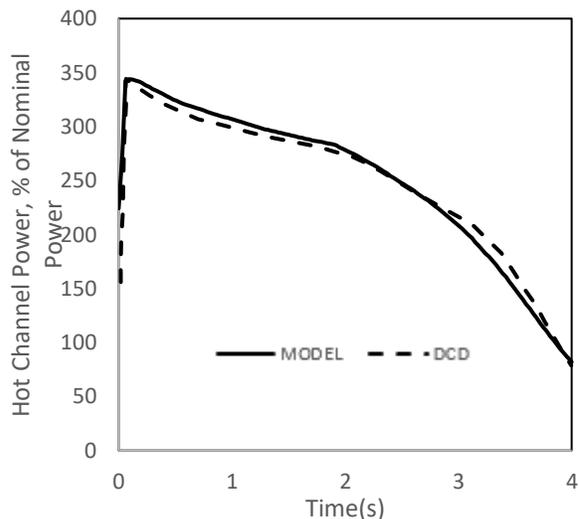
**Figure 5:** Hot channel power comparison between DCD and simulation
