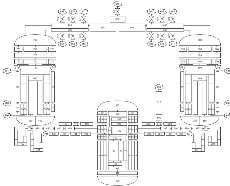
**Figure 2:** System Nodalization
