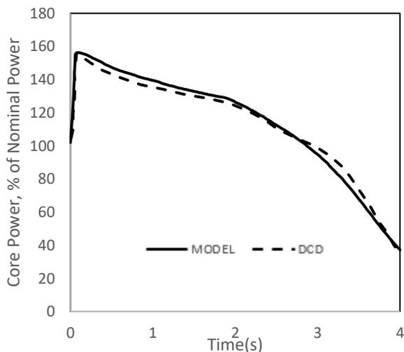
**Figure 4:** Core power comparison between DCD and simulation
