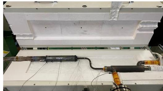
Fig. 6. Experimental facility for the transient test of a bended heat pipe
