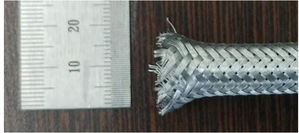
Fig. 2. A schematic of braided wire wick
