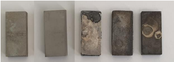
Figure 2. SS316 specimens after exposure to molten chloride salt purified by thermal, Mg, Al, Zn, and Zr, respectively.
