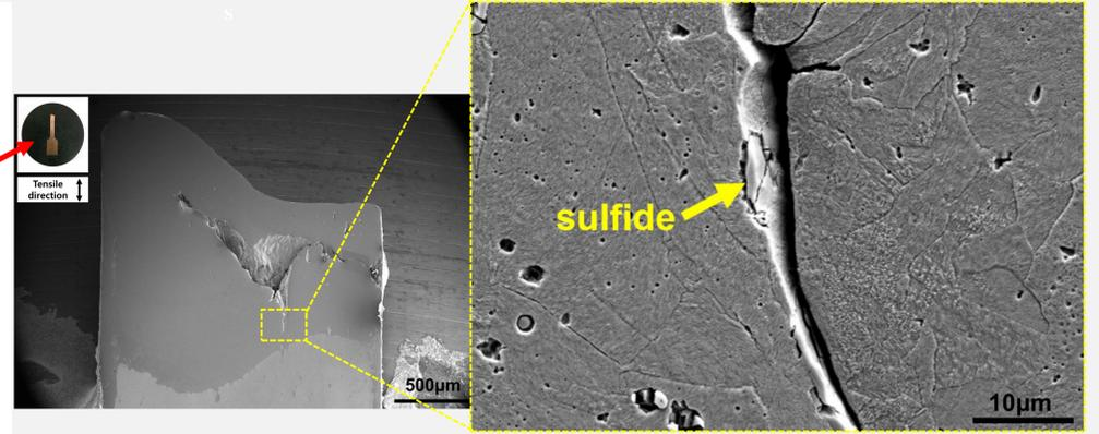
Sulfide on crack tensile fracture of Cu-0.2S SEM image
