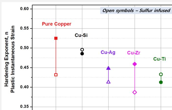
Hardening exponent, n-value of designed copper alloys
