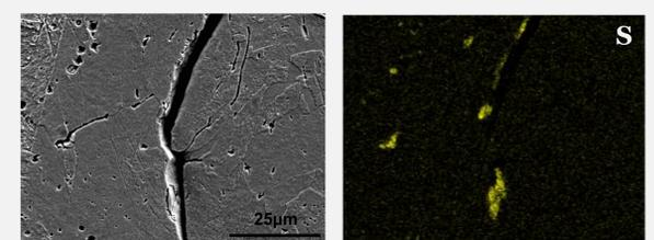
Crack & Precipitate EDS mapping image of Cu-0.2S
