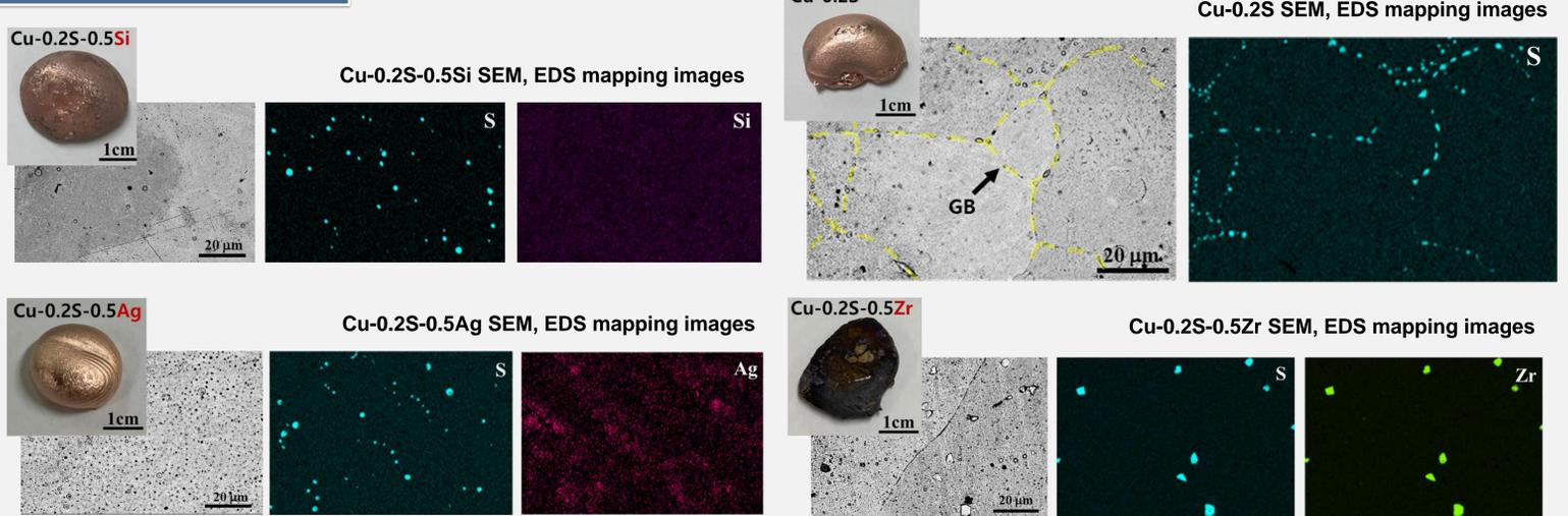
In the case of the casting alloy Cu-0.2S, sulfide was formed on the grain boundary as a result of EDS mapping analysis. For Cu-0.2S-0.5Si, Si is electrochemically dissolved while sulfide is randomly positioned. In the case of Cu-0.2S-0.5Ag, sulfide was formed around the Ag rich phase, and in the case of Cu-0.2S-0.5Zr, sulfide formation energy was lower than Cu, and thus Zr sulfide was formed.
