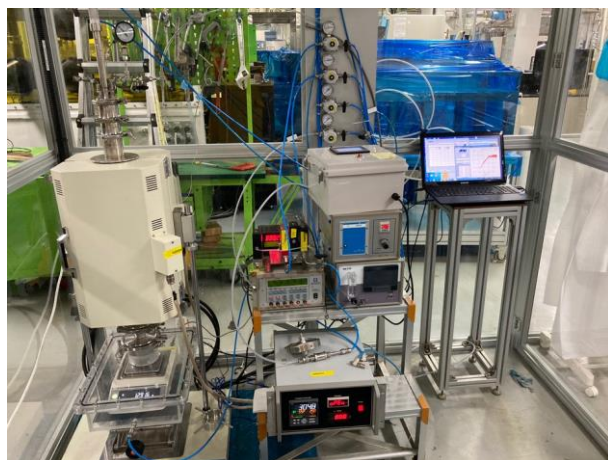
Fig. 1. Air-cylinder based oxidative decladding equipment
