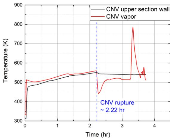
Fig. 4. CNV inner wall averaged surface temperature and CNV vapor temperature.
