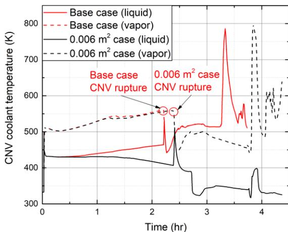
Fig. 8. CNV coolant temperature in 0.006 m<sup>2</sup> flooding case and base case.
