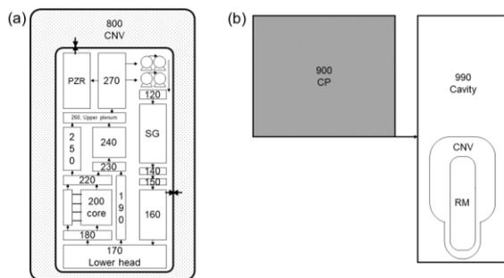
Fig. 2. MELCOR nodalization (a) reactor pressure vessel and containment vessel of ATOM, (b) flooding safety system.
