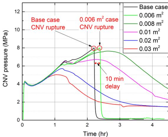
Fig. 7. CNV pressure in flooding cases and base case.
