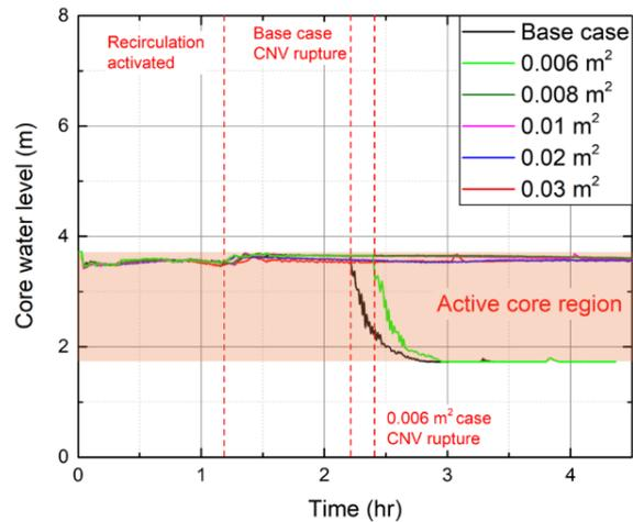
Fig. 9. Water level of CNV and core in flooding case and base case.
