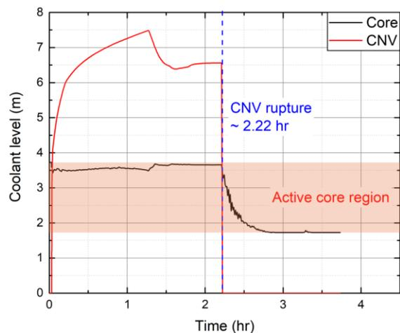
Fig. 5. Coolant level of core and CNV.
