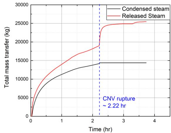
Fig. 6. Total mass of released steam into the CNV and condensed steam on the CNV wall.
