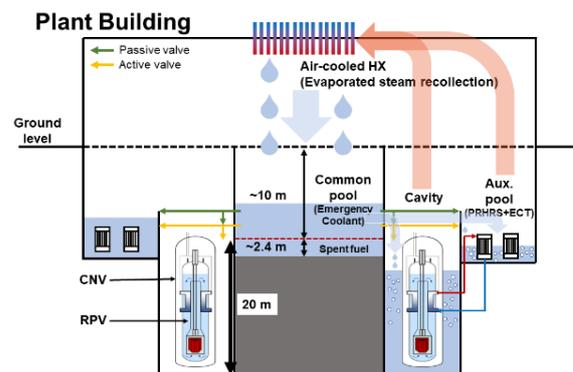
Fig. 1. A conceptual schematic of FSS.
