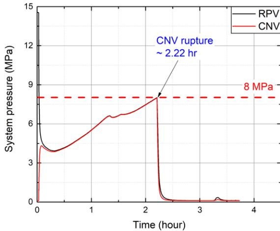
Fig. 3. System pressure of RPV and CNV.
