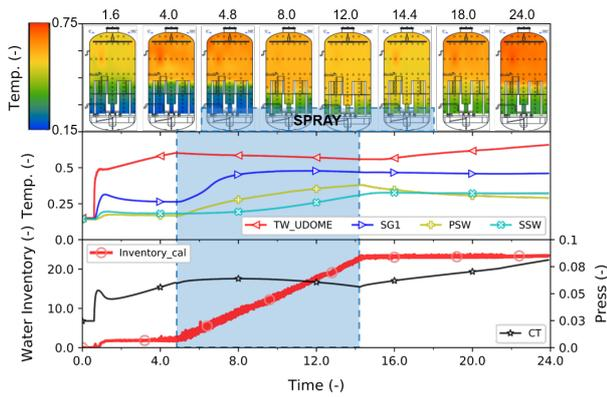
Fig. 3 Comparison of containment thermal-hydraulics in the SLB-CT-05 test
