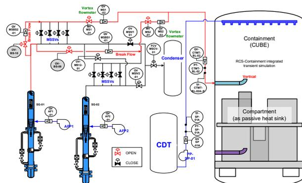
Fig. 1 A schematic diagram for the ATLAS-CUBE integrated test
