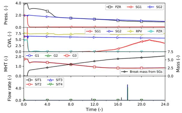
Fig. 2 Comparison of RCS thermal-hydraulics in the SLB-CT-05 test
