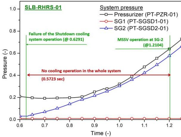
Fig. 3 System behavior after SCS operation failure
