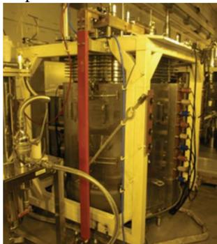
Fig. 4. Photographs of electrolytic reducer with a capacity of 50 kg/batch installed in PRIDE (KAERI) [11].
