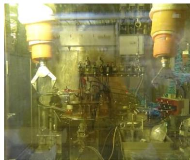
Fig. 3. Photographs of electrolytic reducer installed in M8 hot cell (KAERI).
