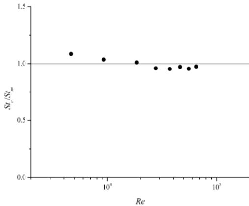
Fig. 4. Variation of  $St_c/St_m$  according to the  $Re_D$  by Eq. (24).
