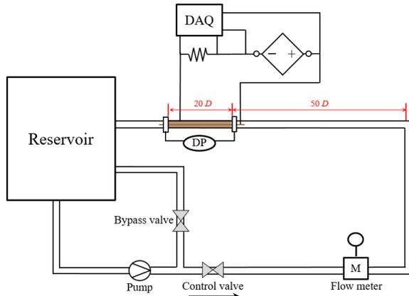
Fig. 1. Schematic diagram of forced convection loop.
