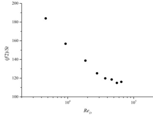
Fig. 2. Variation of  $(f/2)/St$  according to the  $Re_D$ .
