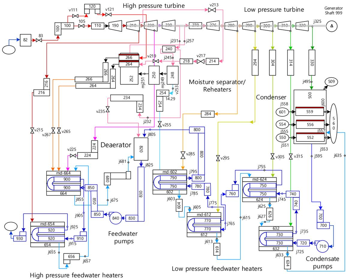
Fig. 1. MARS-KS modeling of secondary system
