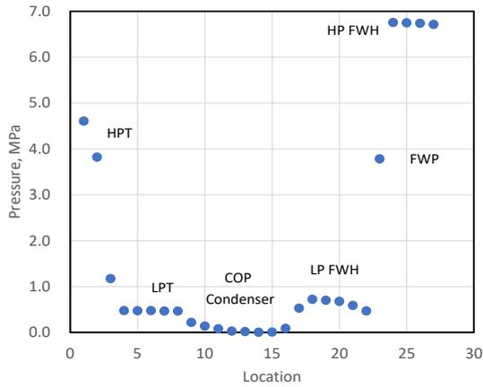
Fig. 2. Calculated pressure distribution
