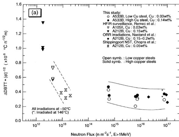
Fig. 3. Normalized increases in ductile-to-brittle transition temperature as a function of neutron flux, defined as increase in ductile-to-brittle transition temperature divided by a square root of the neutron fluence [7].
