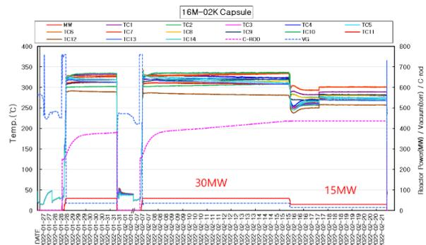
Fig. 2. Temperature variation of specimens during an irradiation testing of the 16M-02K capsule (102-2 cycle).
