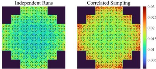
Fig 7. Relative standard deviations of power distribution on 650 EFPD from independent runs (left) and correlated sampling (right)
