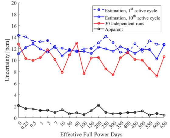
Fig 5. Burnup-dependent  $k_{eff}$  standard deviation
