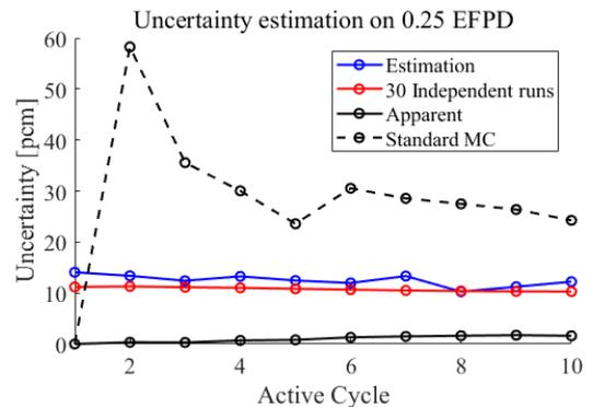
Fig 6.  $k_{eff}$  standard deviation on first burnup step
