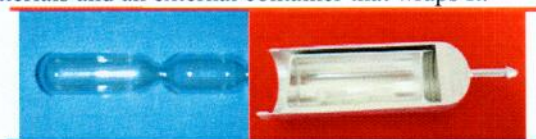
Fig. 1. Target ampoule for neutron irradiation
