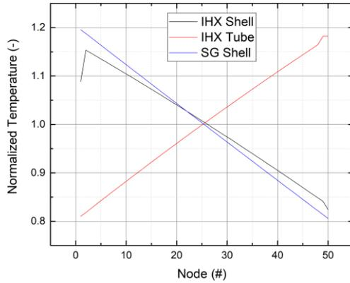
Fig. 3. Temperature change in IHX and SG
