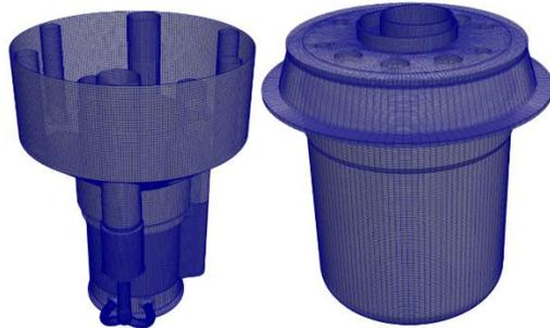
Fig 5. Grid systems of the inner (left) and the outer (right) region of the reactor
