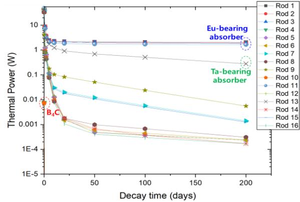
Fig. 4. The decay heat evaluation result after 224 EFPD irradiation
