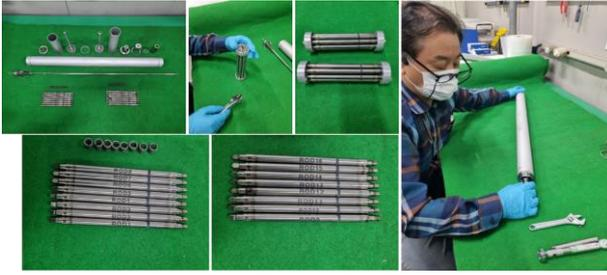
Fig. 3. Assembling test rig with test rods
