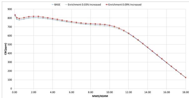
Fig. 8. Burnup calculation results of fuel enrichment adjusted
