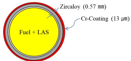
Fig. 2. Schematic of LAS doped with Cr-coating fuel.
