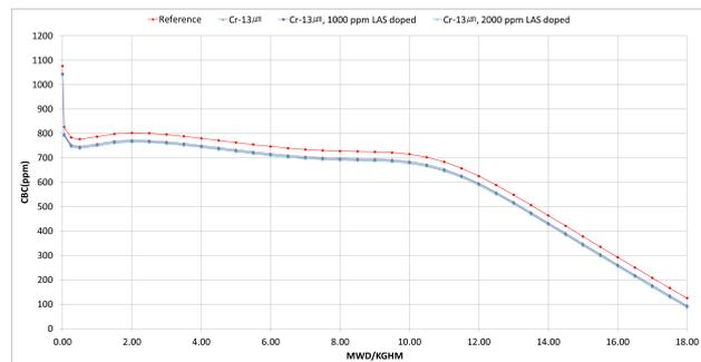
Fig. 7. Burnup calculation results of LAS-doped, Cr-coated condition
