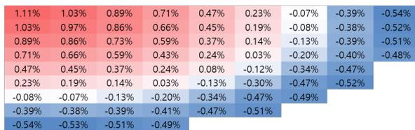
Fig. 4. Power distribution difference (13 μm Cr-coated)
