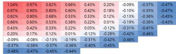
Fig. 5. Power distribution difference (1000 ppm LAS doped)
