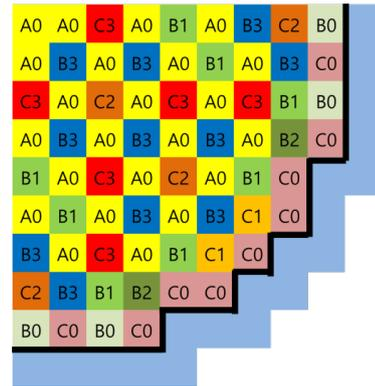
Fig. 1. APR1400 2D core configuration.
