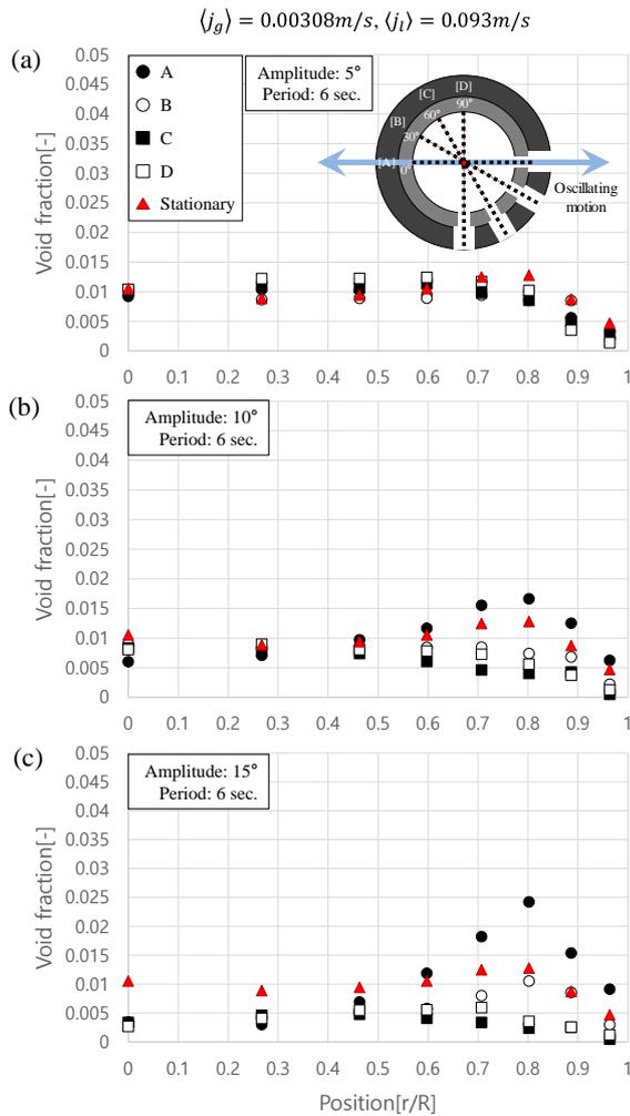
**Fig. 3.** Radial profiles of the time-averaged void fraction at local points under various rolling oscillations (Case 1).
