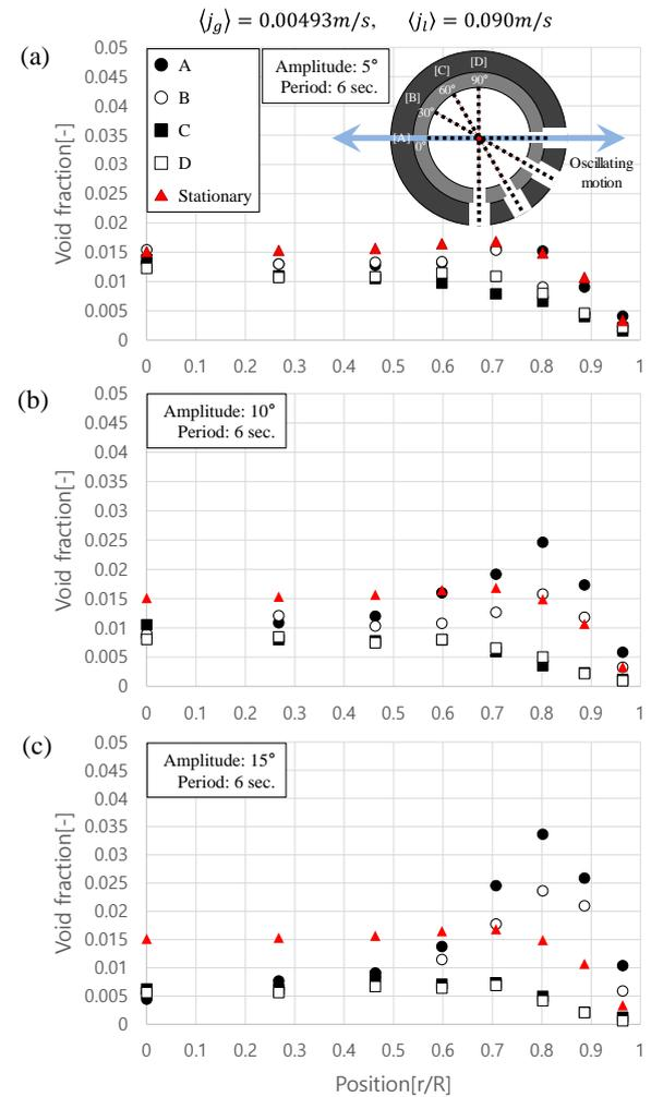
**Fig. 4.** Radial profiles of the time-averaged void fraction at local points under various rolling oscillations (Case 2).
