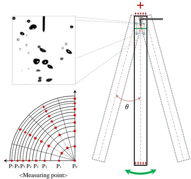
Fig. 2. Experimental conditions: oscillating motion and measuring positions.
