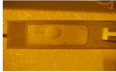
Fig. 6. Fuel plate with blister after heating
