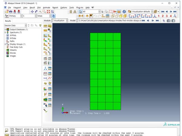
Fig. 2. FE model for the analysis of a two-dimensional flat plate subjected to a simple bending load.
