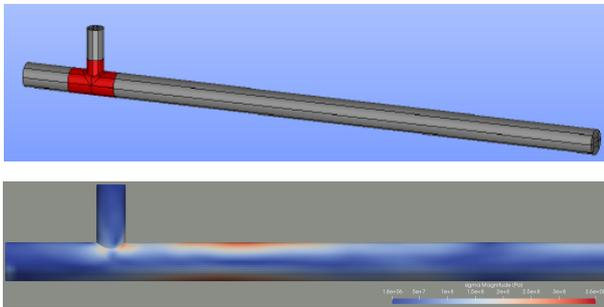
Fig. 3. Coupled FSI analysis model for a T-junction
