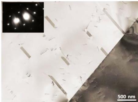
Fig. 2. TEM BF image of stacking faults and dislocations in the austenitic 316 SS before proton irradiation.
