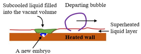
Fig.1. Demonstration of a new embryo, bubble departure, and subcooled liquid occupied the vacant volume
