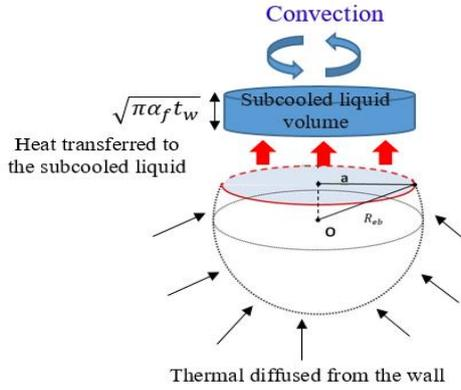
Fig. 3: The heat transfer mechanisms at the nucleation site within the waiting time
