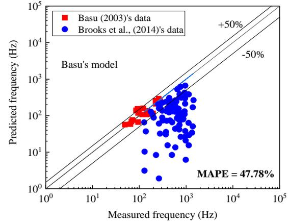
Fig.5: Comparing the predictions of Basu's model with experimental data
